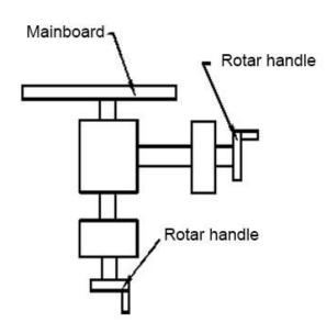
After adjustment of the protection fence, adjust the two turning handle as shown in the below picture, according to the height and position of labeling that the object can be labeled and pass through, and try to adjust to have a stable and smooth movement.
